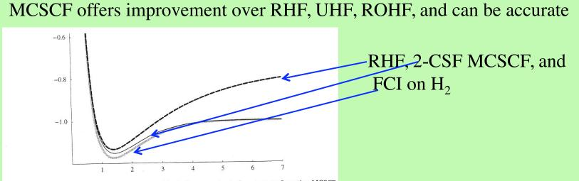
**Fig. 5.14.** The cc-pVQZ potential-energy curve of the hydrogen molecule for a two-configuration MCSCF wave function (solid line) compared with the potential-energy curves of the FCI wave function (thick grey line) and the RHF wave function (dashed line). Atomic units are used.
