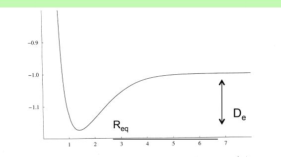
**Fig. 5.9.** The FCI/cc-pVQZ potential-energy curve of the hydrogen molecule in the  $X^1 \Sigma_g^+$  ground state (atomic units).
