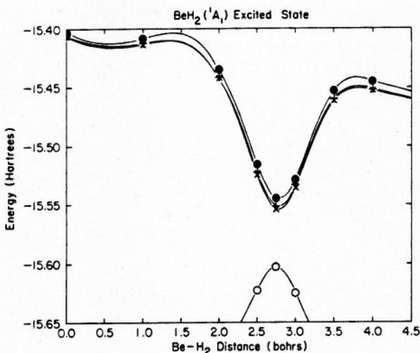
Fig. 1. BeH<sub>2</sub> energies along the path defined in the text. ○: full CI ground-state energy; ★: full CI excited state energy; +: CCMC excited state energy; ●: 18-configuration MC SCF excited-state energy.
