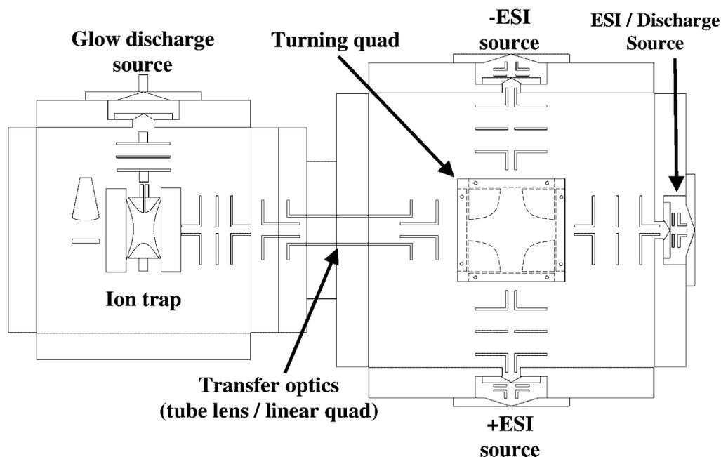
**FIGURE 5.** Schematic diagram of multiple-source quadrupole ion trap mass spectrometer. Adapted from Badman et al., *Anal Chem* 2002, 74, 6237–6243. Copyright 2002 American Chemical Society.
