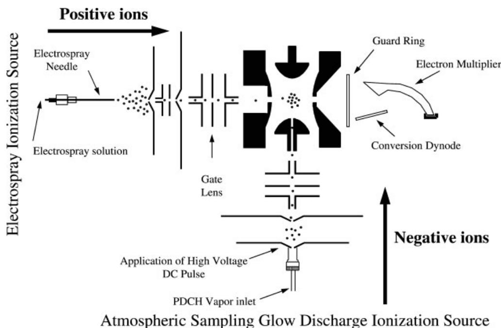
**FIGURE 2.** Schematic diagram of quadrupole ion trap mass analyzer that allows for reactions between ions generated by electrospray ionization (through the end cap electrode) and atmospheric sampling glow discharge ionization (through the ring electrode). Reprinted from *The Encyclopedia of Mass Spectrometry*, Vol. I, McLuckey SA, Ion-ion reactions, pp 866–877. Copyright 2003 with permission from Elsevier.
