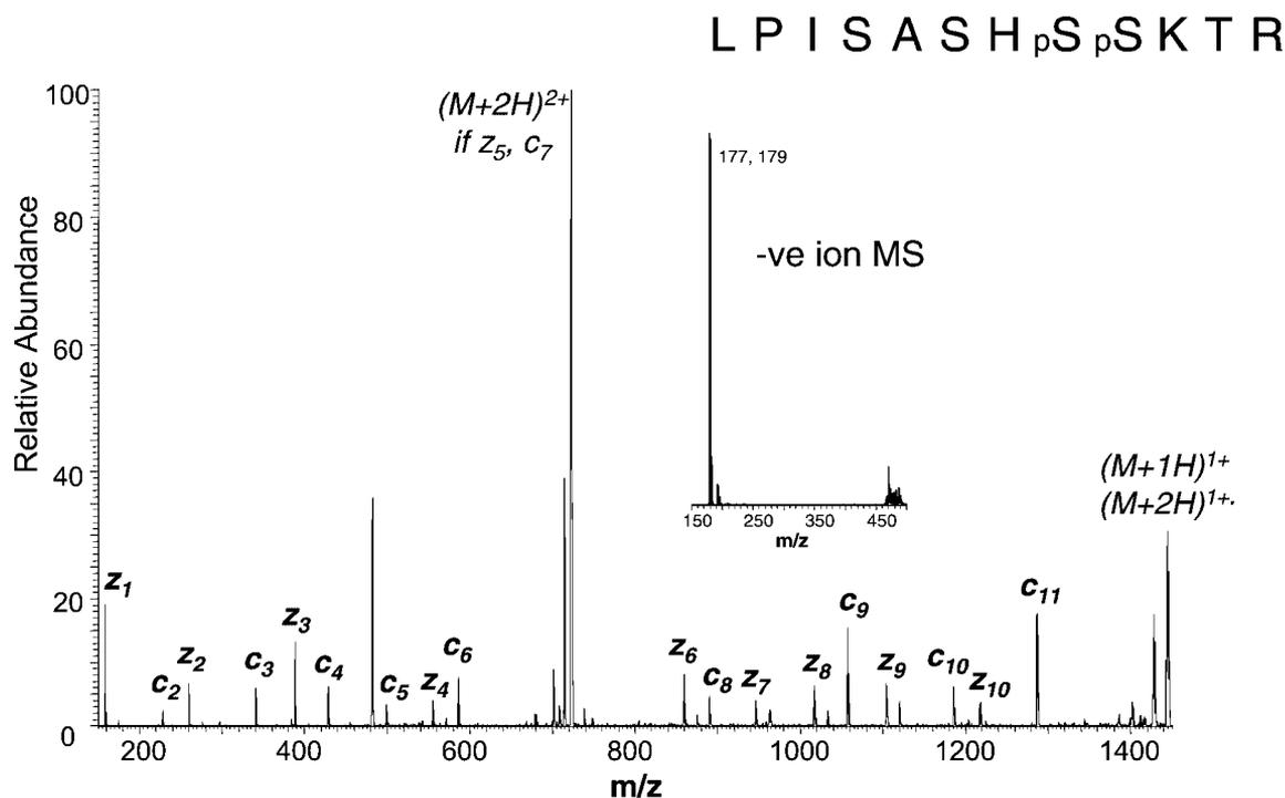
**FIGURE 7.** Electron transfer dissociation mass spectrum of a phosphorylated peptide resulting from ion/ion reactions with  $m/z$  179 anions derived from chemical ionization of anthracene with methane gas (negative ion mass spectrum shown in inset). Figure courtesy of Syka J, Coon J, Shabanowitz J, and Hunt D of the University of Virginia.
