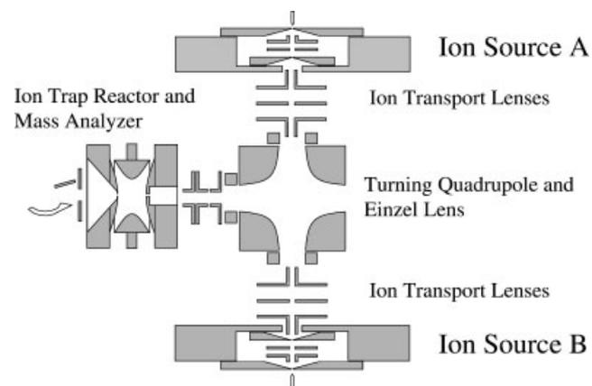
**FIGURE 4.** Schematic diagram of dueling electrospray quadrupole ion trap mass spectrometer Reprinted from *The Encyclopedia of Mass Spectrometry*, Vol. I, McLuckey SA, Ion-ion reactions, pp 866–877. Copyright 2003 with permission from Elsevier.
