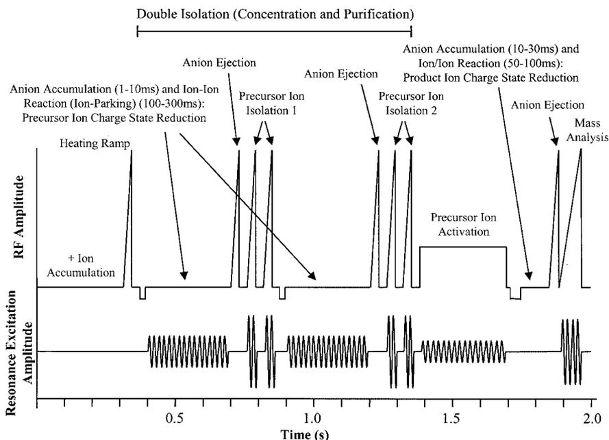
**FIGURE 24.** Schematic diagram of a quadrupole ion trap scan function used in gas-phase concentration, purification, and dissociation of whole protein ions from complex mixtures. Reproduced from Reid et al. with permission from J Am Chem Soc 2002, 124, 7353–7362. Copyright 2002 American Chemical Society.
