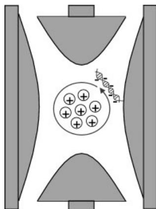
**FIGURE 20.** Representation of trapping by proxy. Positive ions are stored by the electrodynamic ion trap's radio-frequency field. Negative ions are stored by the electric field of the positive ions.
