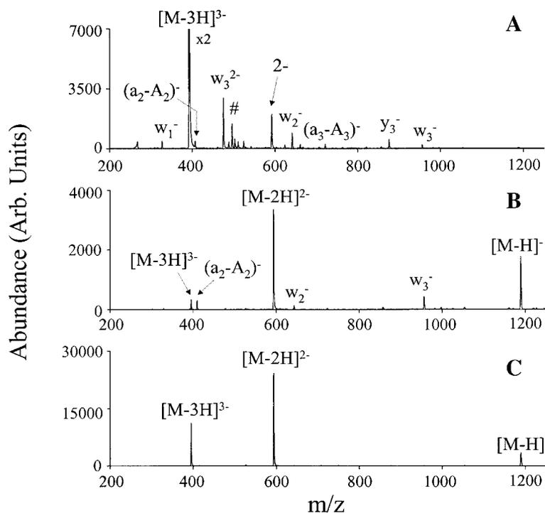
**FIGURE 12.** Ion/ion reaction production spectra of  $[M - 3H]^{3-}$  of 5'-d(AAAA)-3' with (A) O<sub>2</sub><sup>•+</sup>, (B) C<sub>4</sub>H<sub>9</sub><sup>+</sup>, and (C) BQH<sup>+</sup>. # indicates the loss of the terminal base and the terminal sugar. Reprinted from Int J Mass Spectrom, Vol. 228, Wu J, McLuckey SA, Ion/ion reactions of multiply charged nucleic acid anions: Electron transfer, proton transfer, and ion attachment, pp 577–597. Copyright 2003 with permission from Elsevier.
