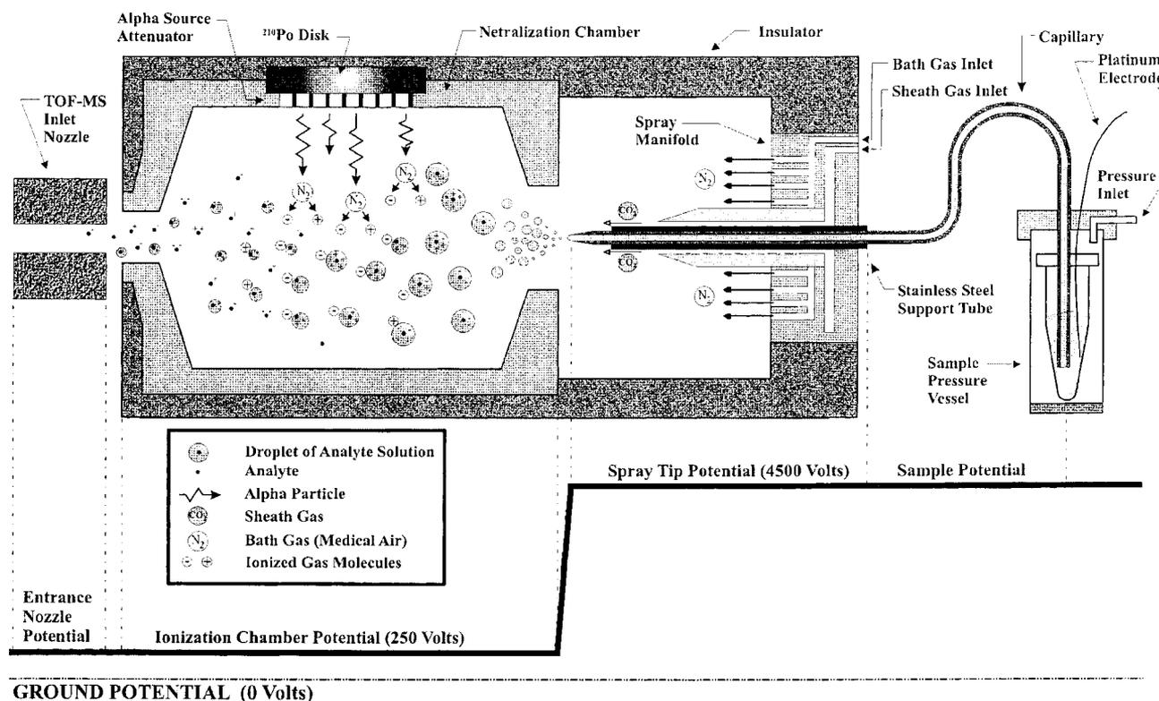
**FIGURE 1.** Schematic diagram of charge neutralization apparatus, which uses  $\alpha$ -particles to reduce the charge of ions formed from electrospray ionization, coupled to a time-of-flight mass spectrometer. Reprinted from Scalf et al. with permission from Anal Chem 2000, 72, 52–60. Copyright 2000 American Chemical Society.
