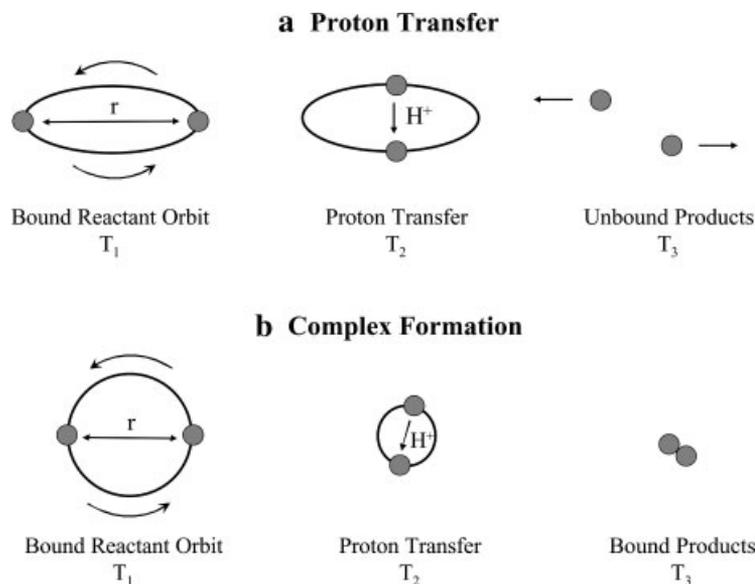
**FIGURE 18.** Schematic representation of the two possible processes resulting from a bound reactant orbit (a) proton transfer (high kinetic energy), and (b) complex formation (low kinetic energy). T = time.
