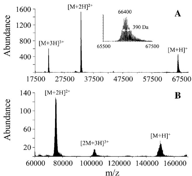
**FIGURE 3.** Post ion/ion reaction mass spectrum of (A) bovine serum albumin, and (B) bovine immunoglobulin IgG. Reprinted from *Int J Mass Spectrom*, Vol. 222, Reid GE, Wells JM, Badman ER, McLuckey SA, Performance of a quadrupole ion trap mass spectrometer adapted for ion/ion reaction studies, pp 243–258. Copyright 2003 with permission from Elsevier.
